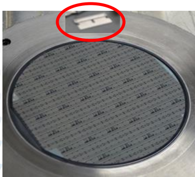
150 mm (6 inch) GaN/Si wafer (Power MOS Fab) with HF/RF/ \mu W HEMT Devices
